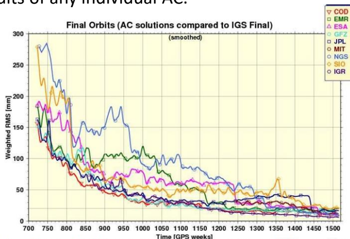
Figure 1: Weighted orbit RMS of the IGS Rapid (IGR) products and AC Final orbit solutions during 1994-2009 with respect to the IGS Final orbit products.
