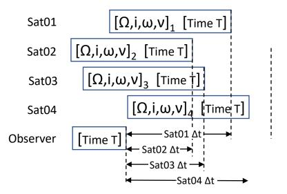
Messages sent at the same time by the satellites are received at different times by the Observer because the signals have to travel different distances. These time differences can be used to calculate those distances. With a knowledge of the satellites' positions and their distance from the Observer, the Observer can calculate its position on the Earth's surface.
